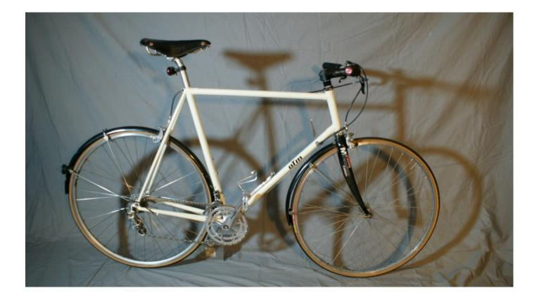
**Description**: Classic Lugged road steel frame with 1" ITM carbon fork and aheadset, BSA 68mm BB. Vintage Campagnolo Record derailleurs and manual 2x9 speed (36x46 Stronglight & 13:25 Campa cassette) gear change (lever on downtube and thumb shifter on handlebar). Rear wheel Mavic Open Pro SUP on Campagnolo Chrorus hub, Single wall alu front wheel. Brooks B17 black leather saddle. SKS fenders
